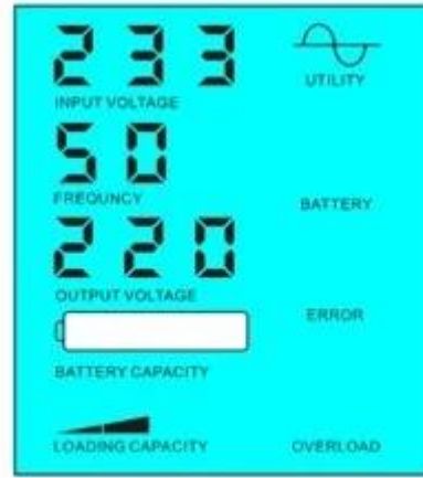
Battery dead, utility supply power
