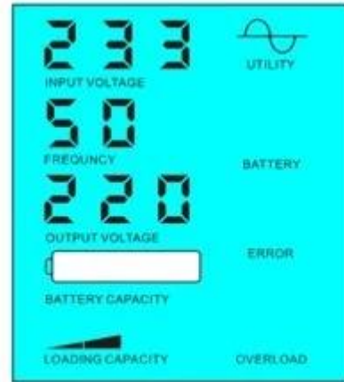
Battery dead, utility supply power
