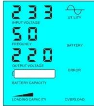
Battery dead, utility supply power
